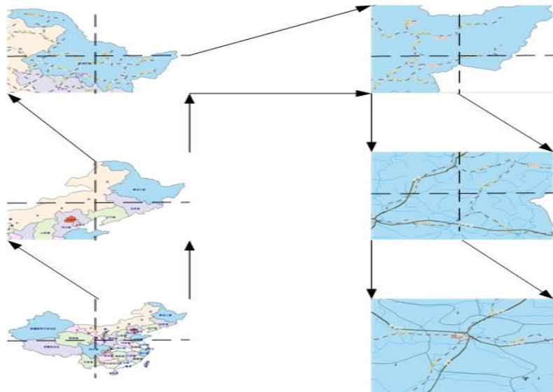
Figure 2. An example of the hierarchical map structure, with each scale being reduced by a factor of four
