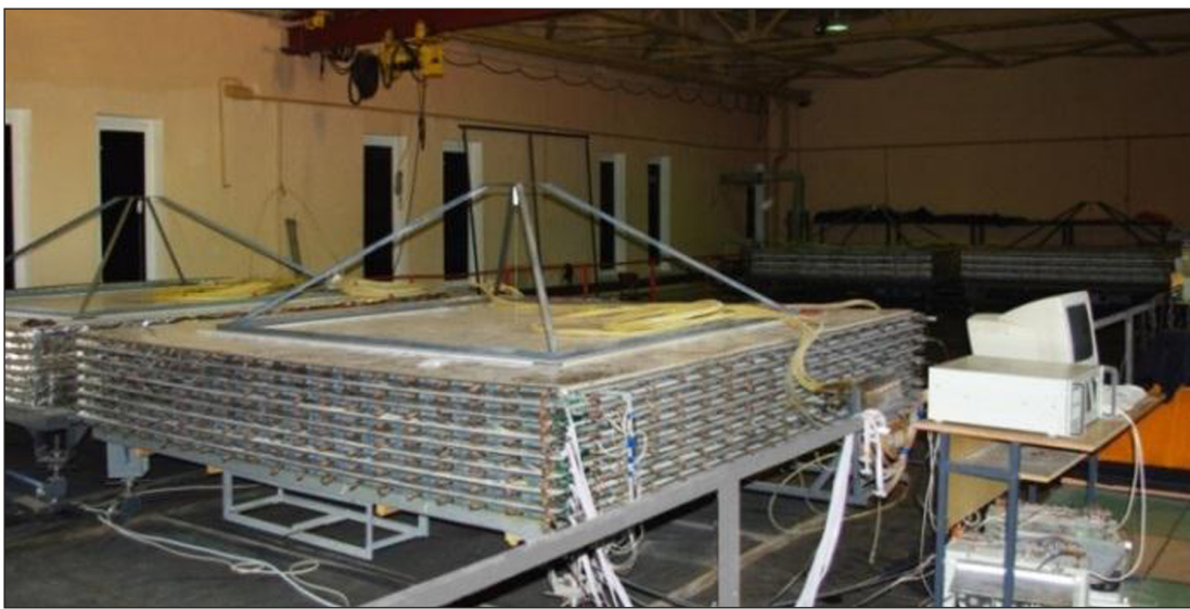
Figure 1: The muon hodoscope URAGAN. In the foreground, one of the supermodules is seen. On the left and at the background the other three SM are located.
